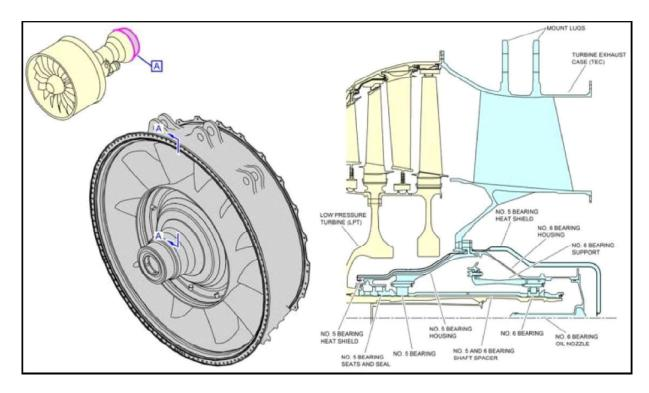
Figure 5: TECM - TURBINE EXHAUST CASE MODULE
