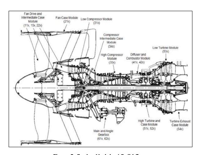
Figure 2: Engine Modules/ Build Group
