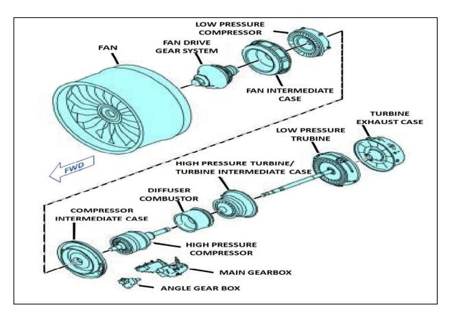
Figure 3: Engine Modules/ Build Group
